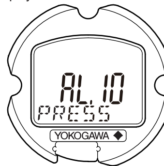
Self-diagnostic error on integral indicator (Faulty transmitter)
