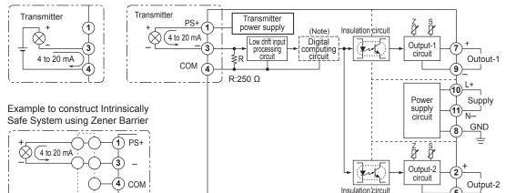
Note: Digital computing circuit is added for the input/output suffix codes other than "A" and "6".
