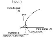
Output signal: DC voltage or DC current signal Output variable range: -6 to 106 % (Both output 1 and output 2)
