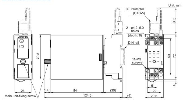
Normal Allowable Deviation= ± (Value of JIS B 0401-2016 tolerance grade IT18) / 2
