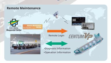
Yokogawa service engineer can remotely log in to onboard CENTUM via VSAT. The operator can make immediate and precise action with Yokogawa consultation. Safest security measures are built-in to the onboard connection.
