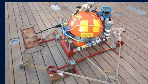
Free-fall pop-up type ocean bottom pressure gauge equipped with the new water pressure gauge used for the evaluation on the seafloor (Provided by: ERI of Tokyo University)
