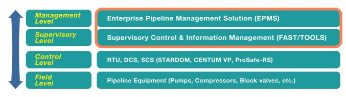
EPMS plugs into the FAST/TOOLS platform and inherits the FAST/TOOLS advantages in one common environment;
