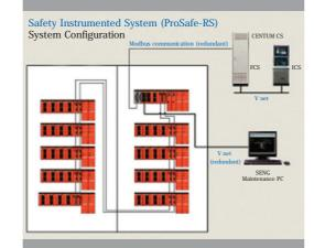
Our ProSafe-RS system has improved reliability by incorporating redundant CPU and I/O modules to avoid unnecessary trips triggered by system abnormalities, not by true safety concerns.
