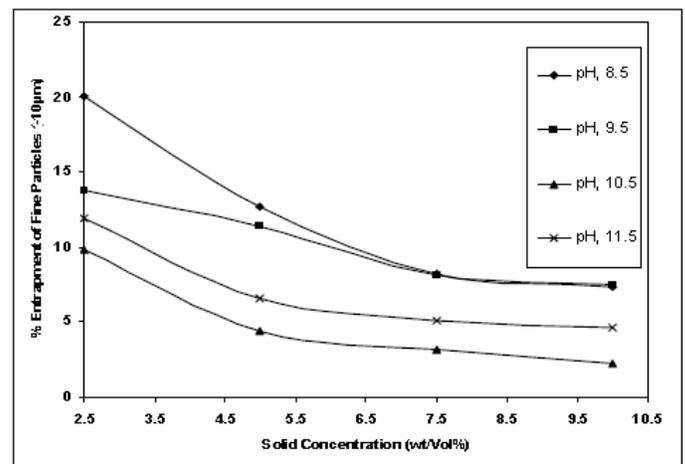
**Figure 2:** Effect of pH and solid concentration on stabilization of -38 µm iron without dispersant.
