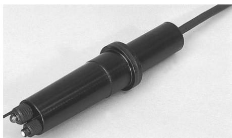
PH8EFP standard Ryton pH sensor is solid electrolyte pH sensor. With the body made of Ryton, a strong engineering plastic, which is comparable to Teflon in terms of corrosion resistance and heat resistance, it allows for a wide range of applications. The integrated-sensor design simplifies calibration with standard solutions and maintenance.
