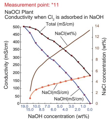
The correlation between concentration and conductivity is largely affected by solution temperature. The ISC inductive conductivity meter provides automatic temperature compensation using the build-in temperature sensor.
