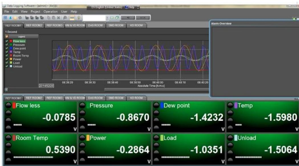
Figure 2 GA10 software monitoring live process values from air compressor
