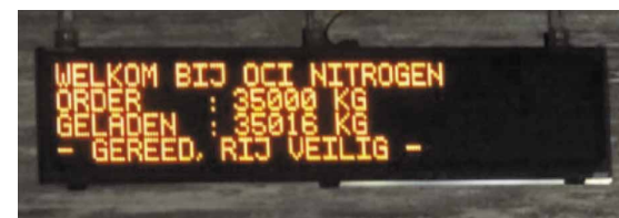
Each bay has a multi-language scoreboard giving guidance to the truck driver on bay assignment, ordered weight, loading progress, etc.
