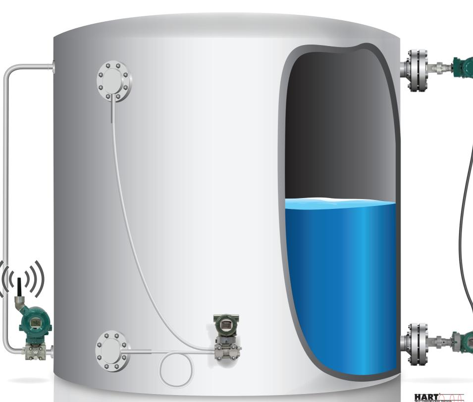
Liquid tank level is one of the basic measurements used in process plants but, its importance cannot be overstated. Incorrect high levels can cause the vessel to overflow leading to lost product, a safety hazard, or an environmental problem (or all three). Incorrect low levels can burn out pumps. Incorrect level measurement can cause problems with inventory control.
