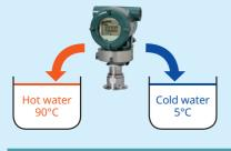
Characteristic when sensor is exposed alternately at 5 to 90°C
