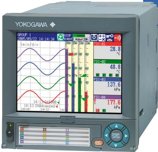
The new DXAdvanced DX1000N features an inner chassis that can be removed from the case via the front panel of the instrument. This provides access to all of the internal components of the DX1000N from the control panel without having to access the rear of the unit or disturb any of the field and power supply wiring. Functionality, appearance, and panel cutout dimensions are the same as those of the standard DX1000.
