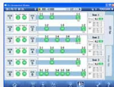
Virtual GCs can also be set up inside a single GC with GCMs to measure multiple streams simultaneously with minimal impact on the complexity of the GC configuration; significantly reducing the project costs. Not only does this reduce the number of GCs needed but it also reduces the size of the analyzer shelter; leading to even more savings. And with the GCM software and display concept, the added complexity of combining GCs into one unit is dramatically reduced.
