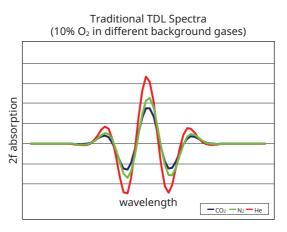
The TruePeak we can measure the area of the absorbance peak. This eliminates effects from changing background gases, allowing for simple pressure and temperature compensation.
