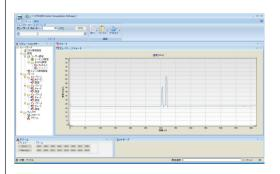
Using the DTAP200 application, you can configure and control the DTSX200, display measured temperature data and generate LAS format data, and remotely perform control, monitoring and analysis anywhere via Ethernet.
