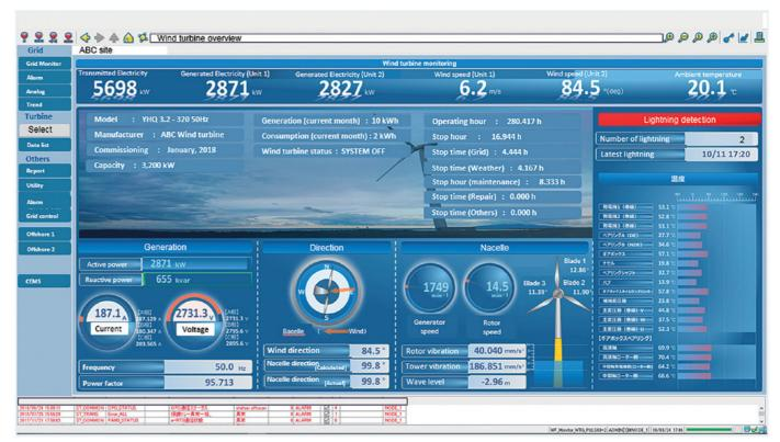
Example display of wind turbine monitoring
