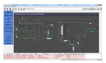
STARDOM allowed for full process control similar to what is expected from a DCS with the lower cost point of a PLC. It also featured tight integration with FAST/TOOLS to allow for rapid screen development and data integrity through data buffering and backfill on network or server outage.
