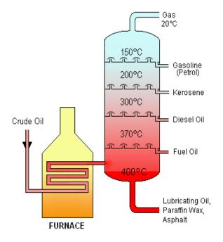
An oil refinery is an industrial process plant where crude oil is processed and refined into more useful petroleum products, such as gasoline, diesel fuel, asphalt base, heating oil, kerosene, and liquefied petroleum gas. The measurement of hydrogen purity throughout a system allows for efficient control of the process.
