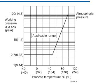
Figure 1-2. Working Pressure and Process Temperature [For EJA530E]
