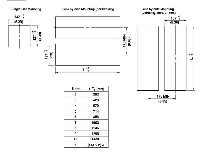
Note: If not specified, the tolerance is  $\pm 3\%$ . However, for dimensions less than 10 mm, the tolerance is  $\pm 0.3$  mm.
