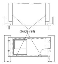
\* For mounting with guide rails, a maintenance space (200 mm or more) should be provided on top of the main unit.
