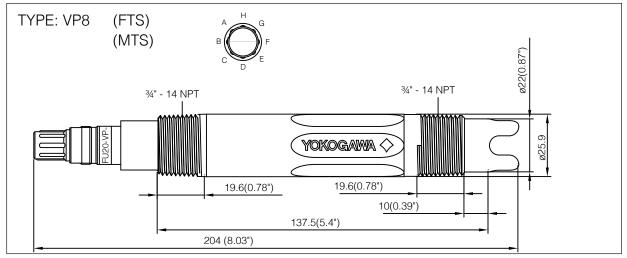
Fig 1. Dimensional drawing FU20-FTS
