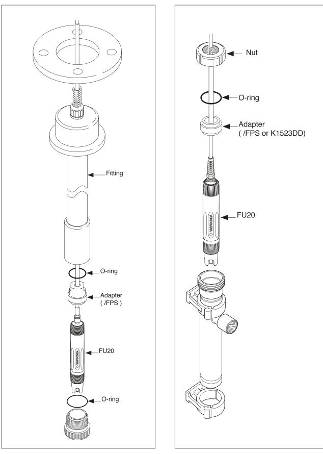
Fig 9. Installation examples for the FU20 in FD40
