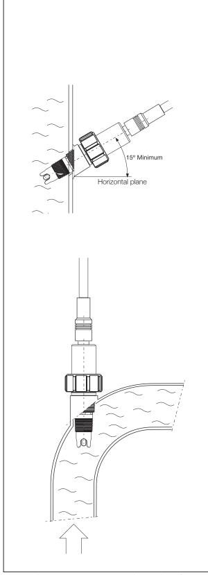
Fig 4. Direct process connection using the ¾" NPT thread using available adapters.
