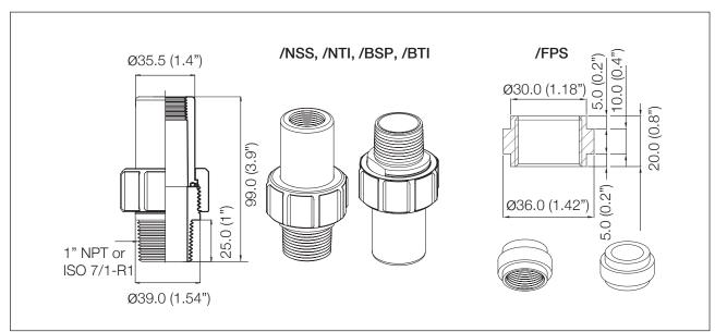
Figure 6. Dimensions 1" FU20-FTS/MTS adapter Stainless Steel & Titanium and FU20-FTS/MTS adapter for FF40, FS40 and FD40 fittings
