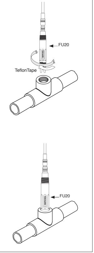
Fig 5. T-piece installation using 3/4" NPT Thread
