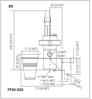
Fig 8. Installation example FU20-FTS/MTS in FF20-flow fitting SS
