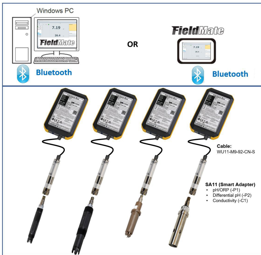
Figure 2: Configuration of IB100 with PC and tablet
