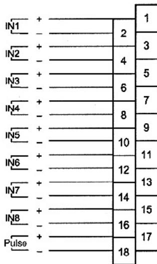
Note: This module is susceptible to noise. Always use shielded cables for wiring. Use an FG clamp on the shield to ground it to a structural metal plate of the module enclosure.
