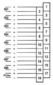
Note: This module is susceptible to noise. Always use shielded cables for wiring. Use an FG clamp on the shield to ground it to a structural metal plate of the module enclosure.
