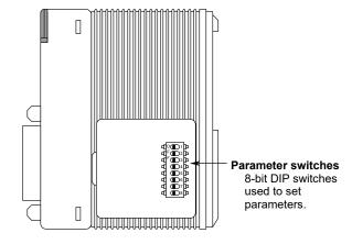
Note: This figure is drawn with the panel cover removed.
