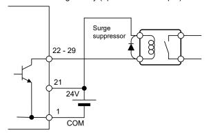
· For connecting an SSR (open collector output)
