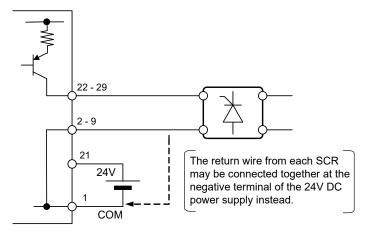
· For connecting a relay (open collector output)
