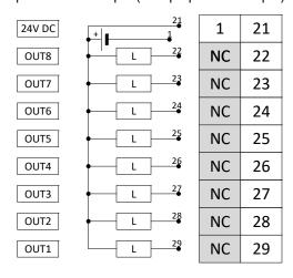
• With OUT1, 3-5, and 7-8 as open collector outputs, and OUT2 and OUT6 as analog outputs
