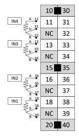
• With IN1 as the thermocouple input, IN2-3 as the RTD input, and IN4 as the DC voltage input
