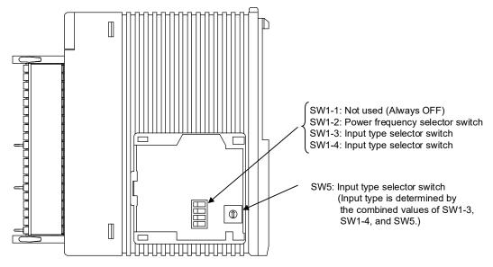
Note: This is the right side view of the module with its cover removed.
