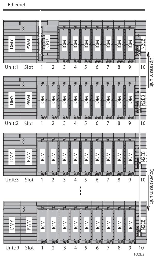
**Example: Control unit with duplexed CPU modules, power supply modules, and E2 bus + 8 extension units / 1 lines**
