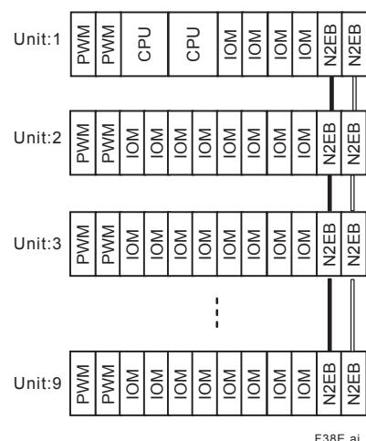
**Example: Control unit with duplexed CPU modules, power supply modules, and E2 bus + 8 extension units / 2 lines**
