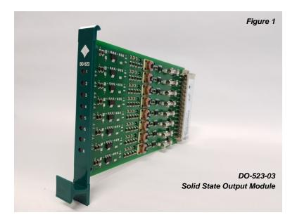
The module converts current pulses to a current sink output. The inputs and outputs are galvanically isolated. Each output is protected with a fuse.
