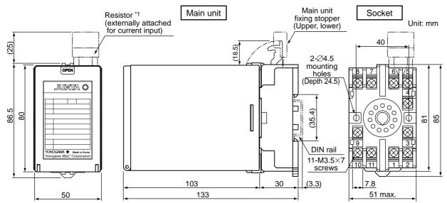
\*1: RES-250 (250  $\Omega$ ) is attached for the input codes A to F, and RES-01K (1k $\Omega$ ) for the input code G.
