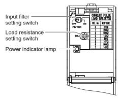
Input filter setting switch: Sets ON/OFF of the input filter.
