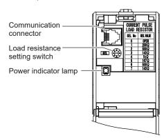
Communication connector: Connect the PC-based Parameter Setting Tool (VJ77). Load resistance setting switch: Sets the resistance value for current pulse input.
