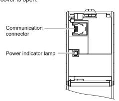
Communication connector: Connect the PC-based Parameter Setting Tool (VJ77). Power indicator lamp: Turns on at power on.
