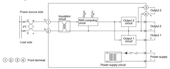
Note: Connect the input signal line to converter-front terminals 1 and 2.
