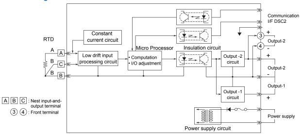
The wiring resistance of input terminals A and B should be the same.
