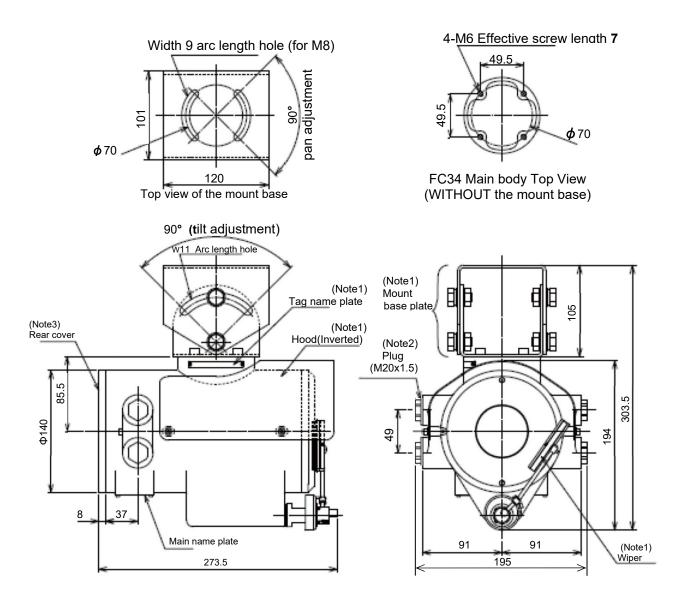
(Note 1): By using each option specification code at the time of order, it will be attached to the product at the time of shipment. (Note 2): A plug is attached to each cable output port for prevention of water leakage into the main body. Please remove the plug before making a connection.
