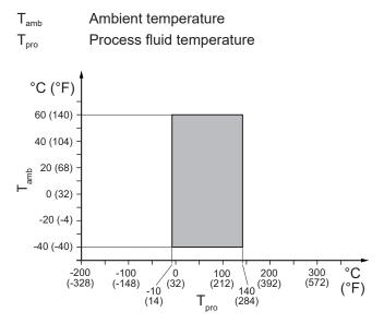
Fig. 13: Allowed process fluid and ambient temperatures, integral type for process connection type HS4 and HS8
