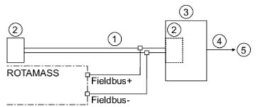
Fig. 36: PROFIBUS PA connection
