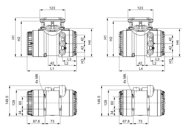
Fig. 18: Dimensions of transmitter in mm
