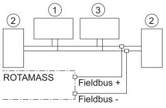
Fig. 37: FOUNDATION Fieldbus connection
