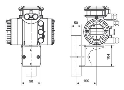
Fig. 19: Dimensions of transmitter in mm, attached to mounting bracket.
