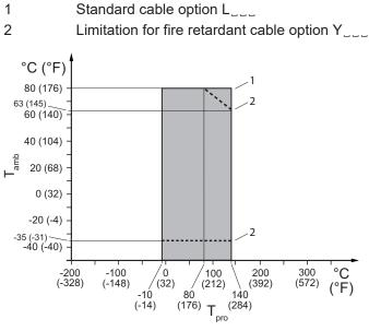
Fig. 15: Allowed process fluid and ambient temperatures, remote type for process connection type HS4 and HS8
