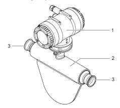
Fig. 2: Configuration of the Rotamass integral type
