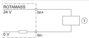
Fig. 23: Connection of external device with passive current output
