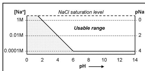
**Figure 2: Application range for the SM23 as a reference electrode in pH measurement**
