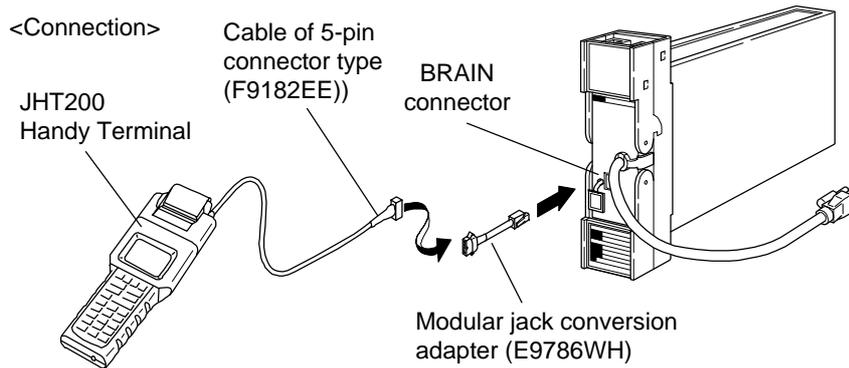
Figure 5-7 Connecting the Handy Terminal
