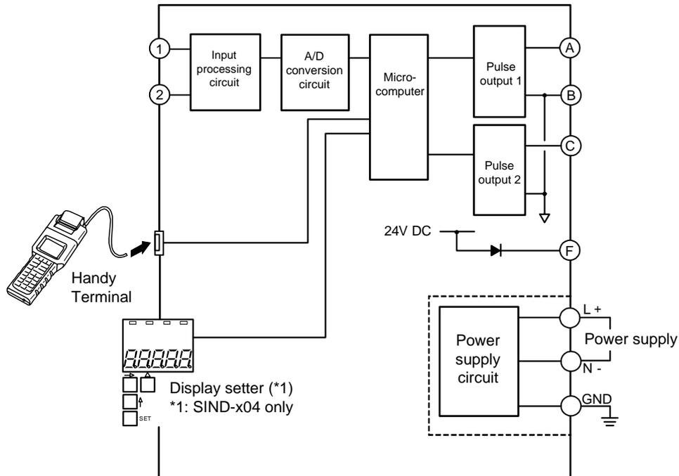
Figure 4-1 Hardware Function Block Diagram
