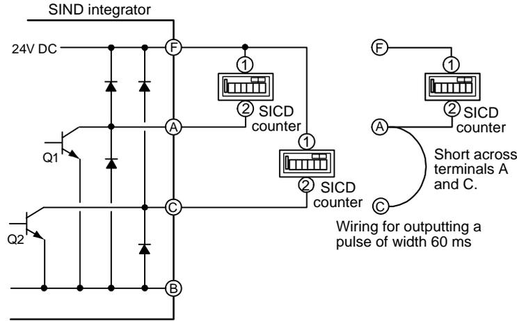
Figure 3-2 Connecting the SICD Counter
