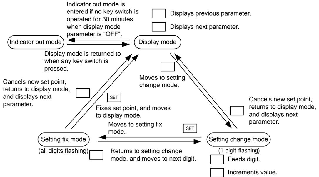
Figure 5-3 Key Switch Operations and Migration of Display States
