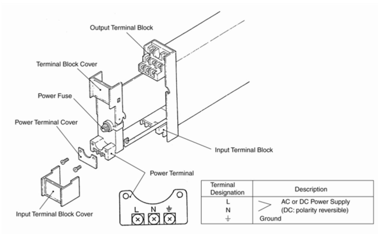
Figure 1 Names of Parts and Power Terminal
