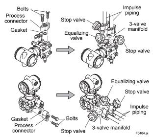
Figure 4.4 3-Valve Manifold (Direct-Mounting Type)
