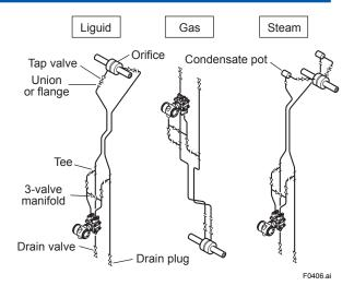
Figure 4.6 Impulse Piping Connection Examples (EJA110A)
