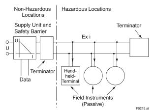
I.S. fieldbus system complying with Entity model
