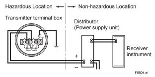
Figure 5.3 Connection between Transmitter and Distributor
