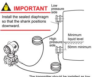
The transmitter should be installed as low as possible below the position where the high pressure side diaphragm seal is installed.
