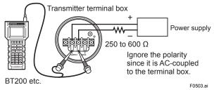
Figure 5.2 Handheld Terminal Connection
