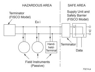
I.S. fieldbus system complying with FISCO model
