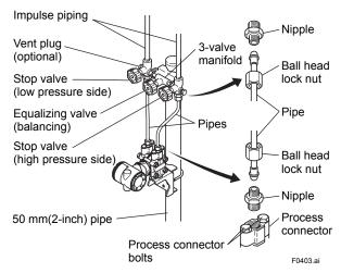
Figure 4.3 3-Valve Manifold (Pipe-Mounting Type)
