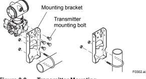
Figure 3.2 Transmitter Mounting (Horizontal Impulse Piping Type)
