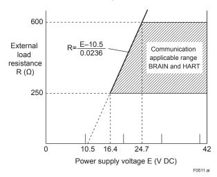
Figure 5.10 Relationship between Power Supply Voltage and External Load Resistance
