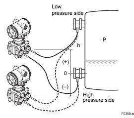
Figure 3.8 Example of Installation to Tank (Caution on Installation)
