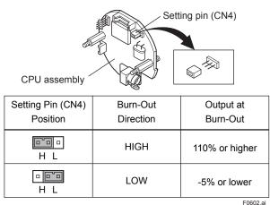
Figure 6.1 Burn-out Direction Setting Pin
