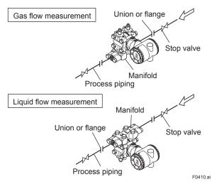
Figure 4.10 Process Piping Connection Examples (EJA115)
