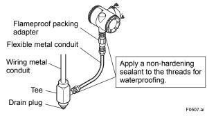
Figure 5.6 Typical Cable Wiring Using Flameproof Packing Adapter
