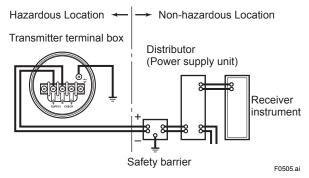
Figure 5.4 Connection between Transmitter and Distributor
