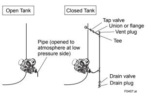
Figure 4.7 Impulse Piping Connection Examples (EJA210A and EJA220A)
