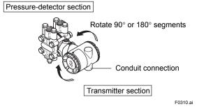
Figure 3.10 Rotating Transmitter Section
