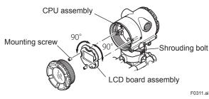
Figure 3.11 Rotating Integral Indicator
