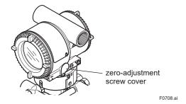
Figure 7.5 Zero-adjustment Screw
