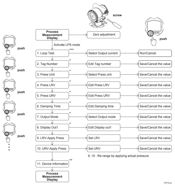
These parameter configurations are available with the software revision (SOFT REV)2.03 or later. Software revision can be checked via a field communicator (HART/BRAIN) or DTM. Please refer to IM 01C25T01 for HART parameter "Software rev" and IM 01C25T03 for BRAIN "SOFT REV."
