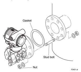
Figure 4.1 Transmitter Mounting
