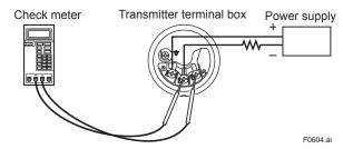
Figure 6.7 Check Meter Connection
