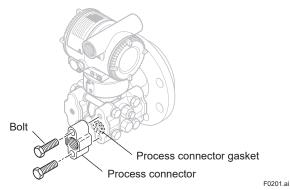
Figure 2.1 Transmitter Mounting Hardware
