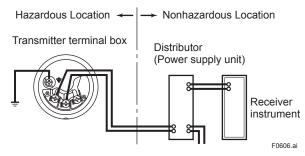
Figure 6.9 Connection between Transmitter and Distributor
