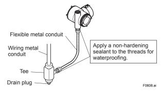
Figure 6.13 Typical Wiring Using Flexible Metal Conduit
