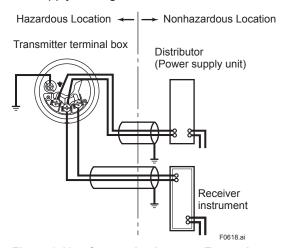
Figure 6.12 Connection between Transmitter, Distributer and Receiver
