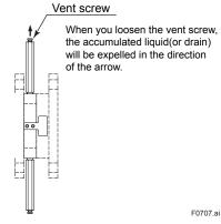
Figure 7.4 Venting for Flushing Connection Ring
