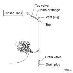
Figure 5.2 Impulse Piping Connection Examples
