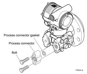
Figure 8.4 Replacing the Process Connector Gasket
