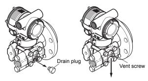
When you loosen the drain plug or the vent screw, the accumulated liquid (or gas) will be expelled in the direction of the arrow.
