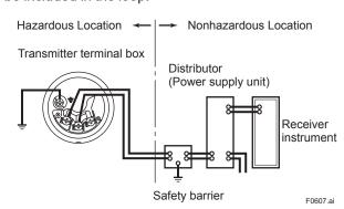
Figure 6.10 Connection between Transmitter and Distributor
