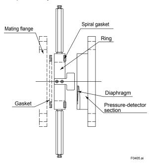
Figure 4.5 Mounting to Process Flange
