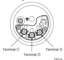
Terminal Wiring for 4 to 20 mA output, FOUNDATION Fieldbus type, and PROFIBUS PA type.
