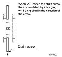
Figure 7.3 Draining for Flushing Connection Ring
