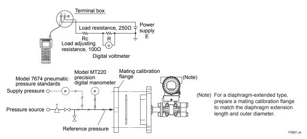
Figure 8.1 Instrument Connections (4 to 20 mA output)
