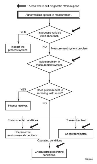
Figure 8.5 Basic Flow and Self-Diagnostics
