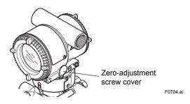
The zero-adjustment screw is located inside the cover.
