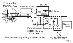
Figure 6.8 Status Output Connection
