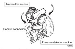
Figure 4.2 Rotating Transmitter Section
