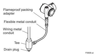
Figure 6.14 Typical Cable Wiring Using Flameproof Packing Adapter
