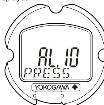
Self-diagnostic error on integral indicator (Faulty transmitter)
