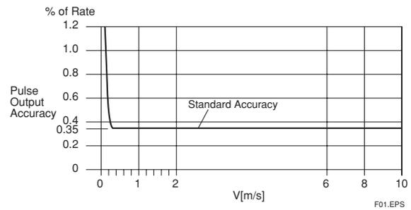
**Current Output "◇":** Pulse output accuracy plus  $\pm 0.05\%$  of Span
