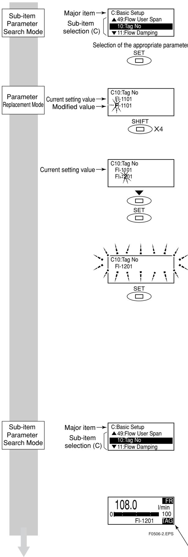
Upon selection of **C: Basic Setup**, the cursor will be positioned at **C10: Tag No**. (Sub-item selection screen (C))
