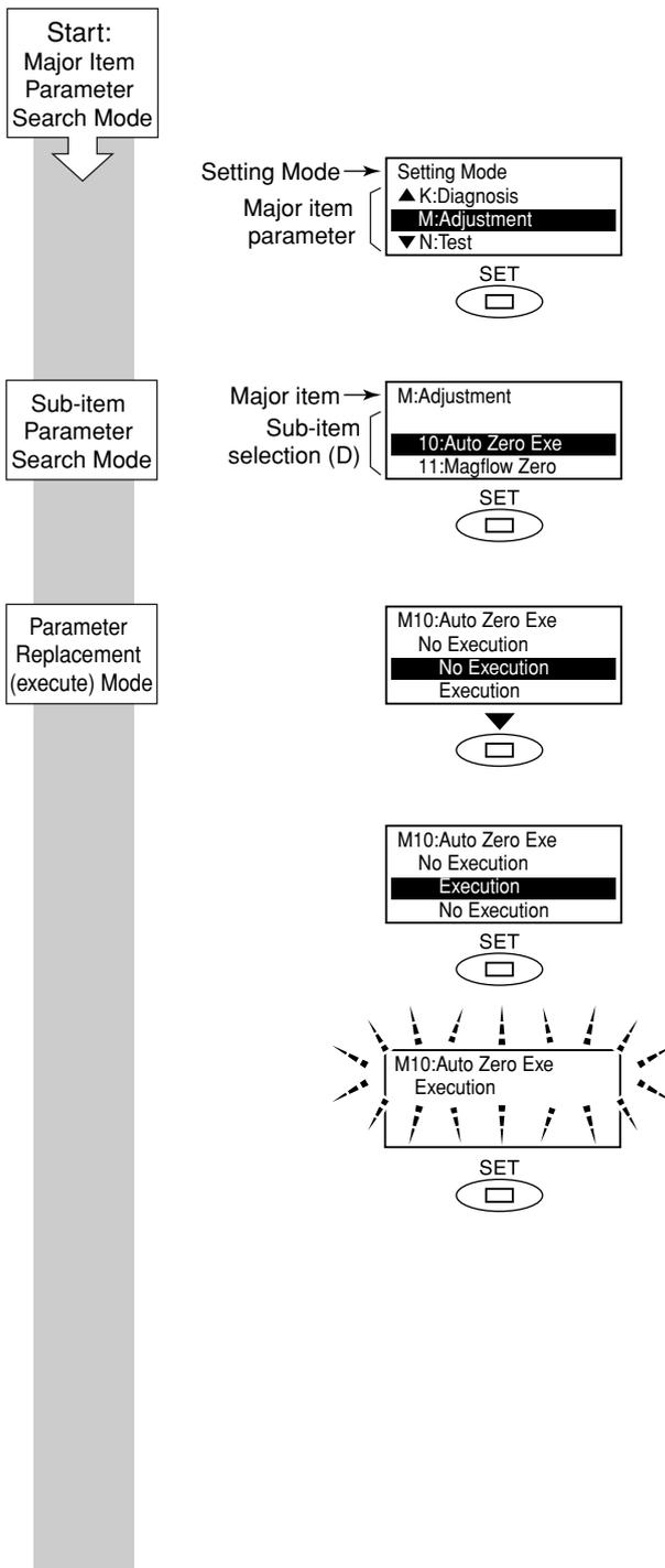
Once in Setting Mode, use the switch to move the cursor to **M: Adjustment**.
