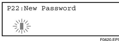
The default setting for this parameter is a string of 8 spaces (i.e., Enable), and thus, the password field will be empty. When the cursor is flashing, the password should be input. Press the SET key twice to confirm the password. The display will then change to “\*\*\*\*\*”.
