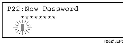
To change a password, first of all use the password originally set with **P21: Enable Wrt Passwd** to release the write protect function, and then set the new password. Alternatively, if it is desired to return to the condition where no password is set, enter a string of 8 spaces.
