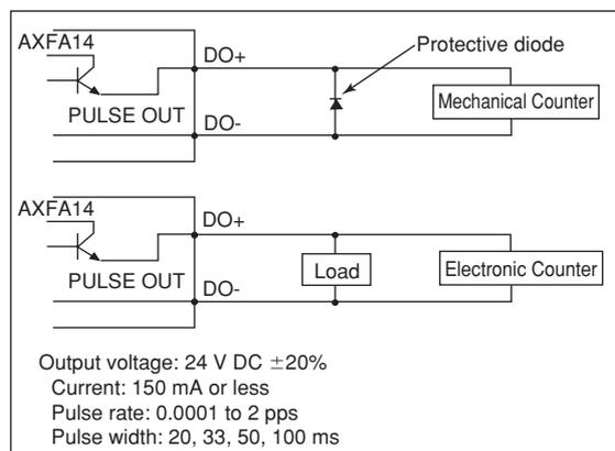
Figure 4.4.9 Active Pulse Output Connection (Optional code EM)
