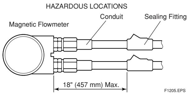
**Figure 12.2 Conduit Wiring****(4) Operation**
