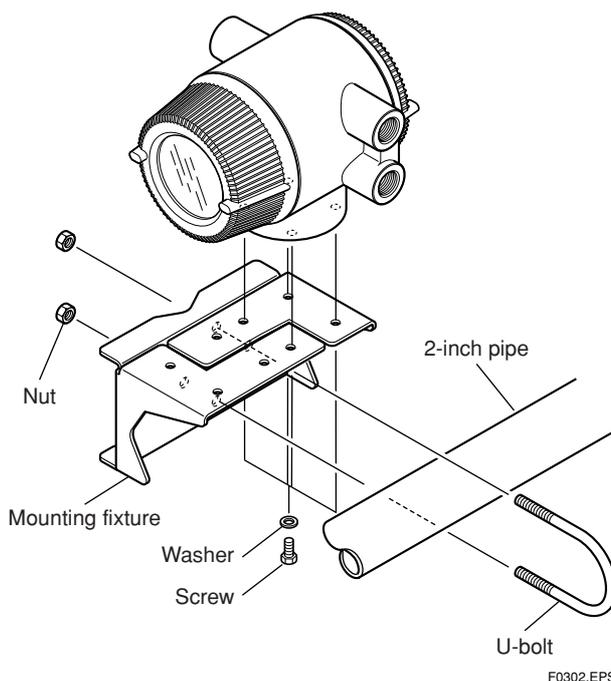
1. Fix the instrument casing on the mounting fixture using four screws.
