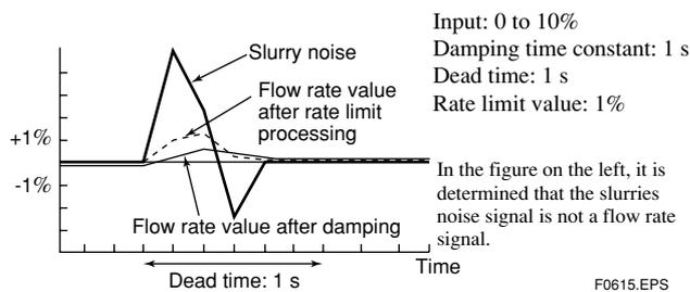
In the figure on the left, it is determined that the slurries noise signal is not a flow rate signal.
