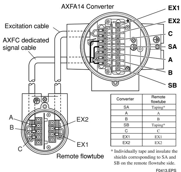
Figure 4.4.5 Wiring Diagram
