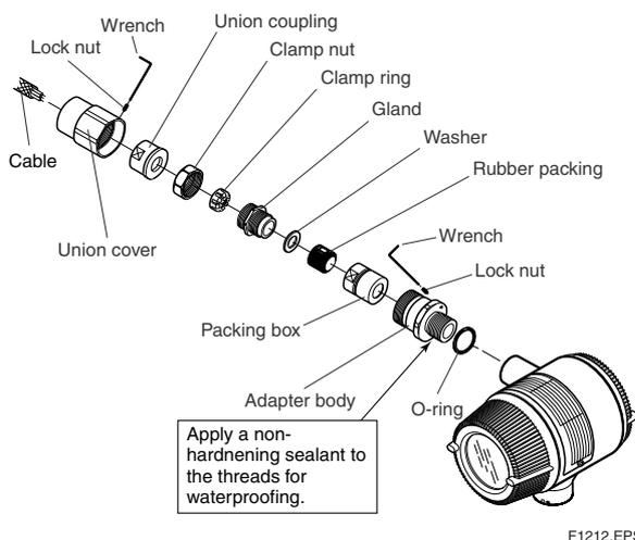
Figure 12.4.3 Installing Flameproof Packing Adapter
