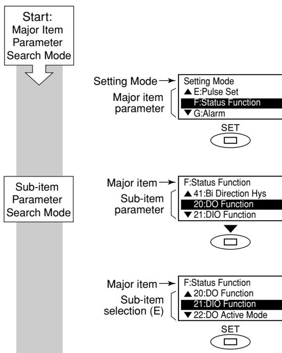
Once in Setting Mode, use the switch to move the cursor to **F: Status Function**.
