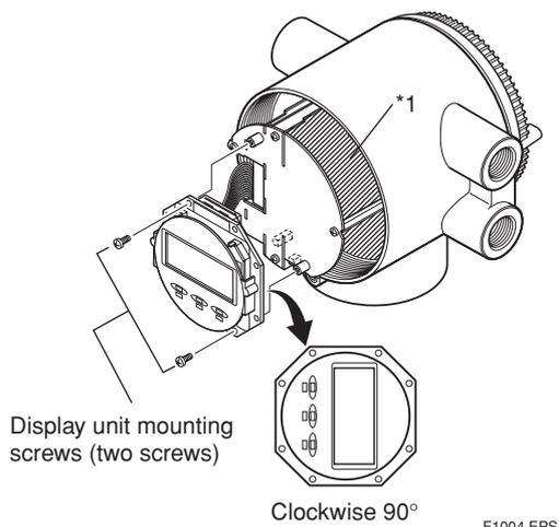
**Figure 10.1.2 Changing the Display Unit Direction 90 Degrees**
