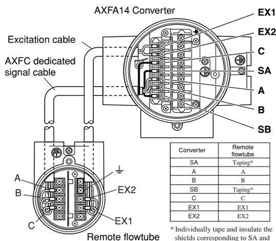
Figure 4.4.6 Wiring Diagram
