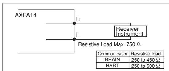
Figure 4.4.7 4 to 20 mA DC Output Connection
