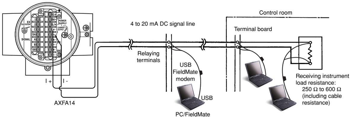
Figure 8.2.1 Interconnection Diagram
