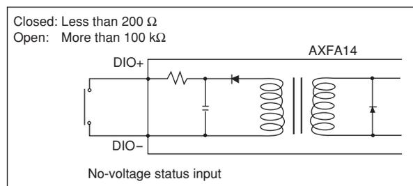
Figure 4.4.10 Status Input Connection
