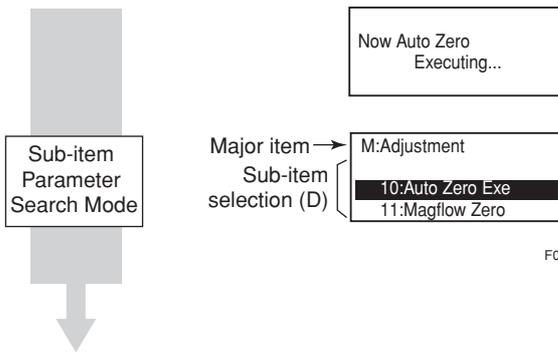
Auto zero adjustment function is being executed (about 30 seconds).
