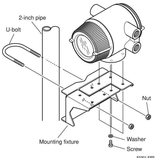
1. Fix the instrument on the mounting fixture using four screws.
