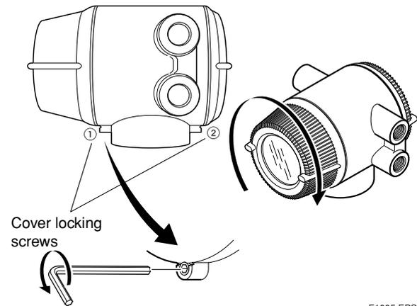
**Figure 10.1.3 Installing the Display Cover**
