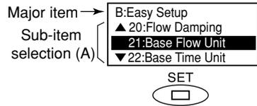
The cursor has been moved to **B21: Base Flow Unit** in this screen. (Sub-item selection screen (A))
