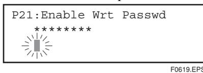
The cursor will flash when entering Parameter Replacement Mode, and the password set with **P22: New Password** should be input at this time.
