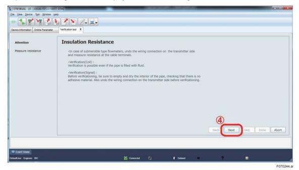
Figure 7.2.44 Continuing Insulation Resistance Check
