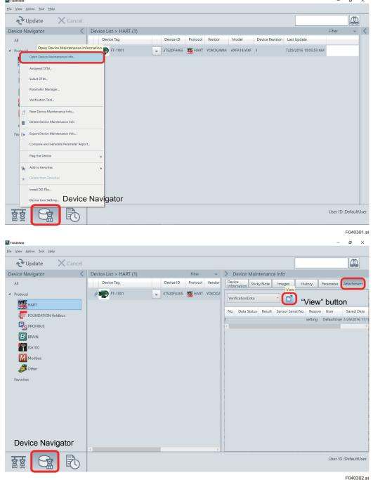
Figure 4.3.1 Start-up from "Device Navigator" by Selecting the "View" Button
