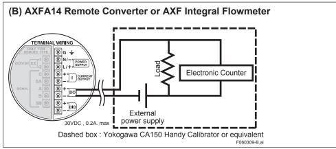
Figure 6.3.9 Pulse Output Diagram (without optional code EM)
