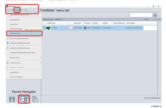
Figure 4.2.2 Start-up from "Device Navigator" by Selecting the "Action" Menu
