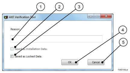
Figure 6.1.6 "Saving Data When "No Flow + Flow" Uncompleted" Dialog
