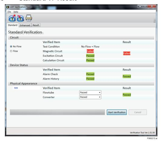
Figure 6.2.13 Example of "Result of Standard VF"
