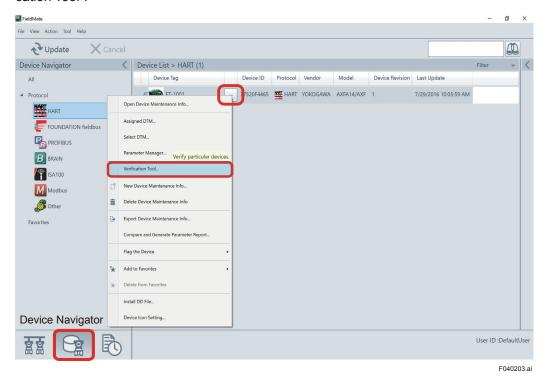
Figure 4.2.3 Start-up from "Device Navigator" by Selecting the "Action" Button
