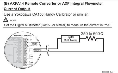
Figure 6.3.3 Current Output Connection Diagram
