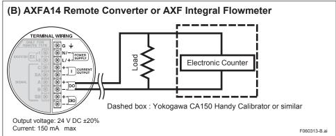
Figure 6.3.13 Active Pulse Output Diagram (with optional code EM)
