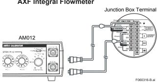
Figure 6.3.16 "Converter" Connection Diagram
